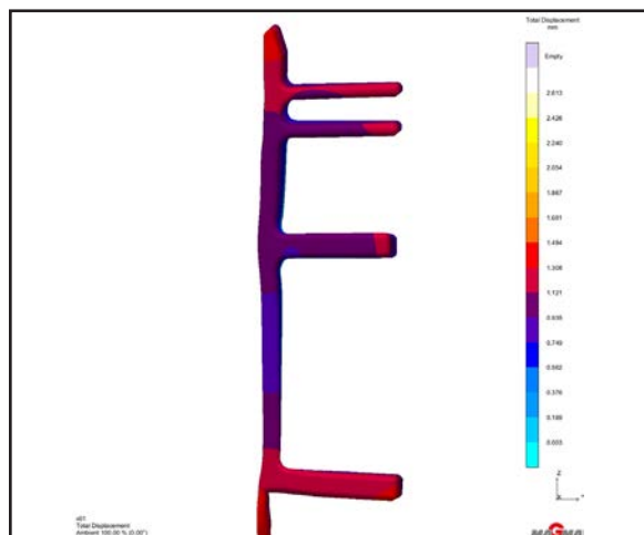
Figure 7-7: Total displacement showing casting shrinkage and distortion with a 25 times scale factor
